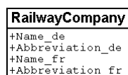
Figure 44: The object class RailwayCompany with names and abbreviations, in German and French respectively.
